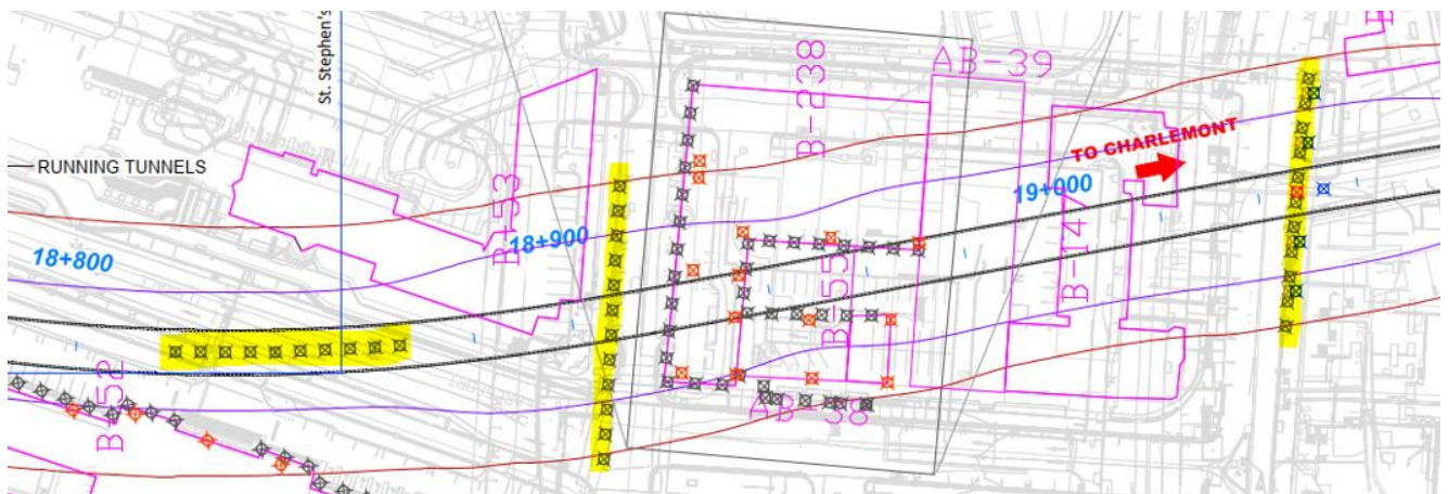
Figure 5-8 St Stephen's Green Tunnel Construction Monitoring – Precise Levelling Points in Roads
