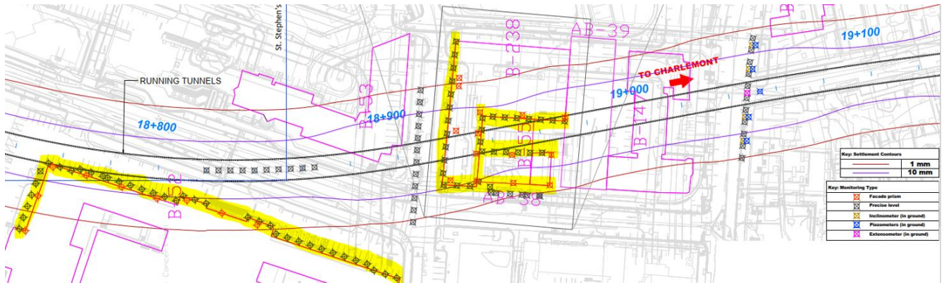
Figure 5-4 St Stephen's Green – Plan of Buildings along Earlsfort Terrace Affected by Tunnel Excavation (including façades requiring fixed monitoring, highlighted in yellow)
